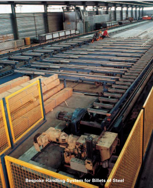
Bespoke Handling System for Billets of Steel
