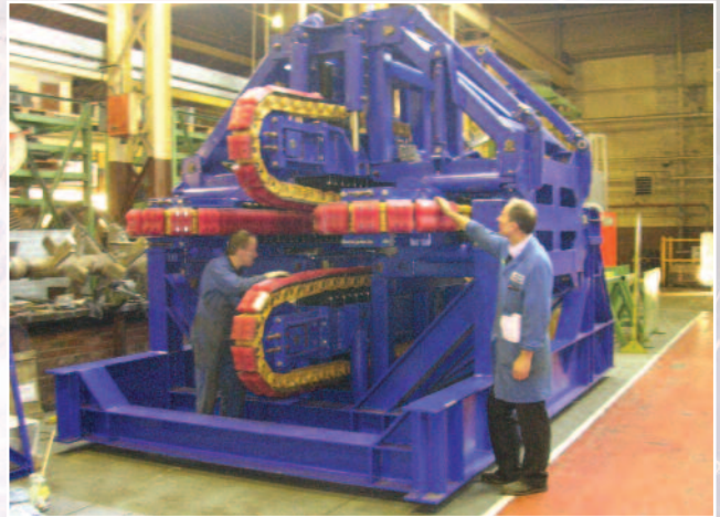
Customer: Baricon Systems Ltd Project: Cable Tensioner Use: Laying cables
