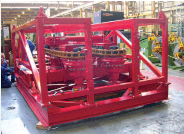
Customer: Baricon Systems Ltd Project: Cable Tensioner Use: Laying cables
