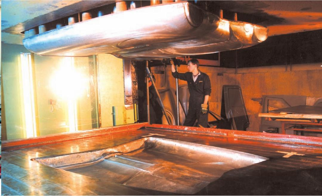
**Main right:** Top and bottom tools manufactured in the Dualform Model 9 press ready for pressing panels.
