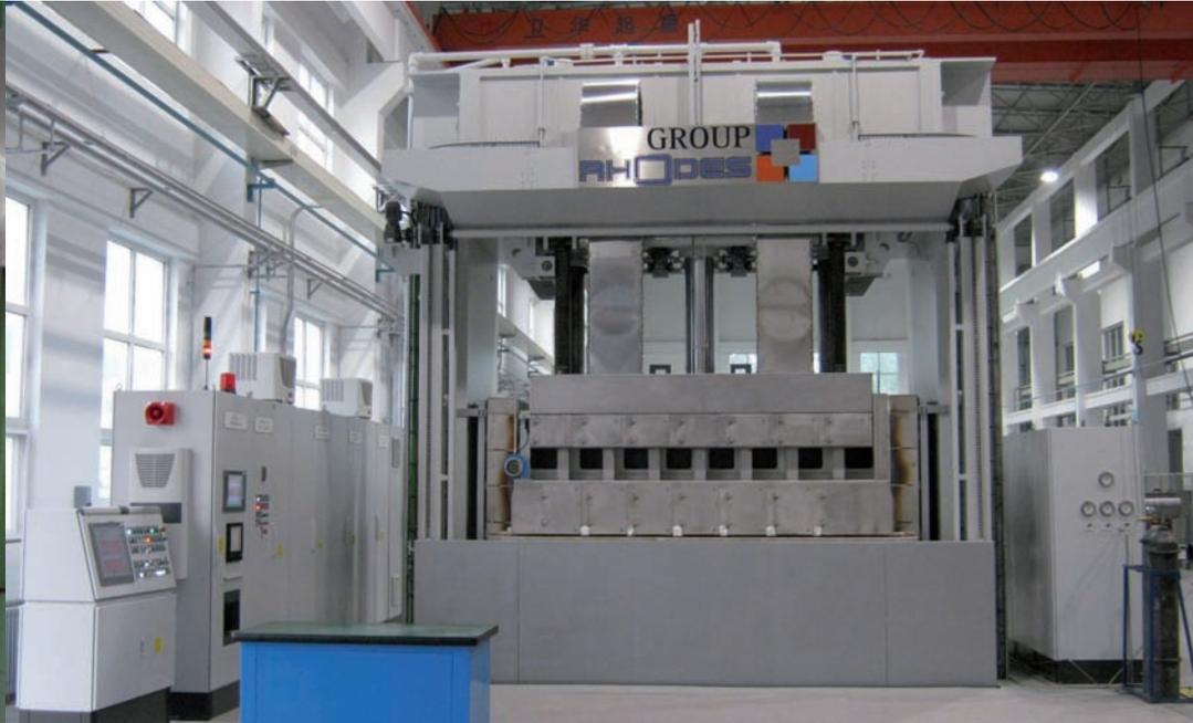
**Main (right):** 1400 tonne SPF/DB press complete with semi-automatic tool loading equipment
