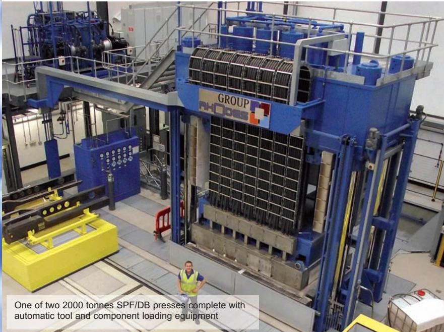
One of two 2000 tonnes SPF/DB presses complete with automatic tool and component loading equipment
