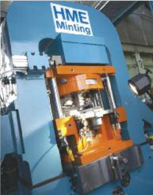
**Above:** Front view of the optional HME fast Hydraulic Tool Clamping System.
