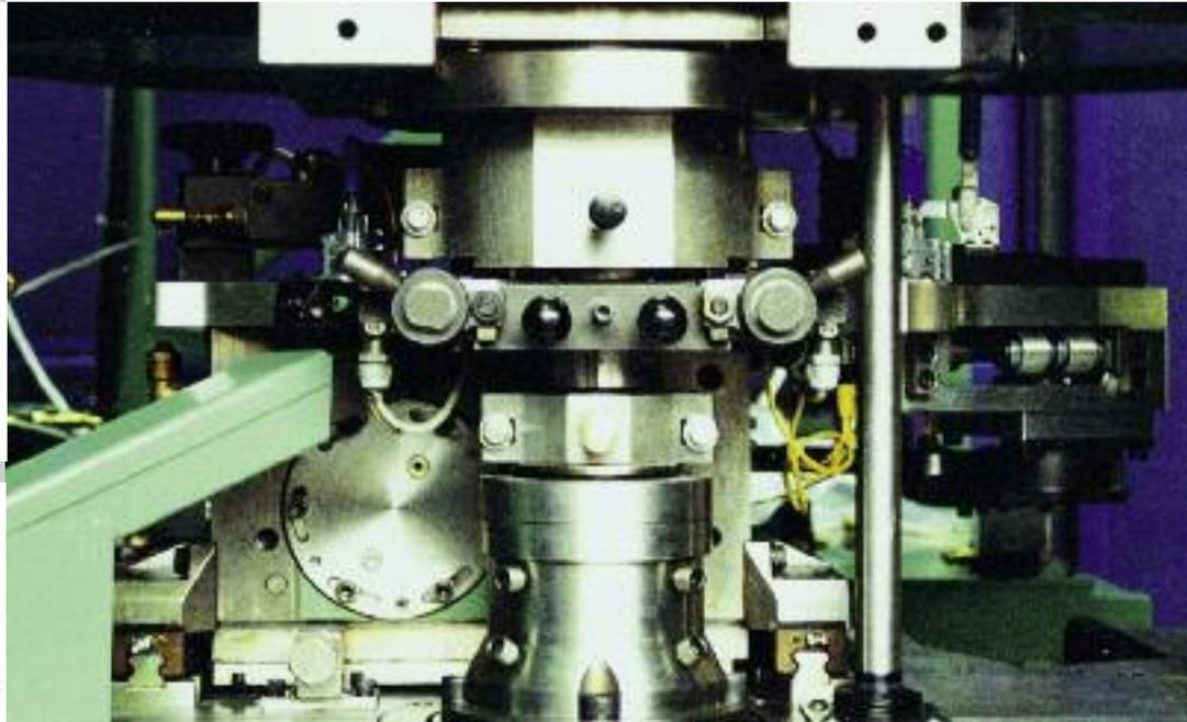
**Main (Right):** Tool area of press showing tooling dies and collars in situ.
