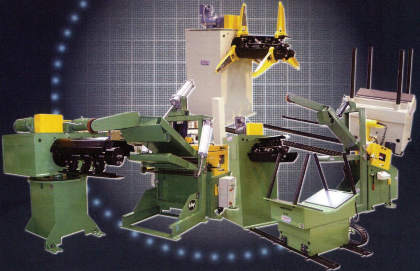
**Coil Loading Cars** - 'V' type coil cars for coils up to 5 tonnes and Mast type for up to 20 tonnes. Coil cars ease coil loading and eliminate waiting time.
