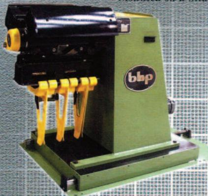
LINK ACTION COILHOLDERS OFFER A COST EFFECTIVE SOLUTION TO COIL HANDLING PROBLEMS. DESIGNED TO HANDLE COIL WEIGHTS UP TO 5000KG. THEY ARE SUITABLE FOR USE IN MOST DECOILING AND RECOILING APPLICATIONS.
