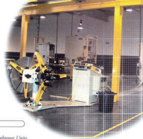
1000kg Double sided Coilholder MS59-300 and RF75-300 Feed Line
