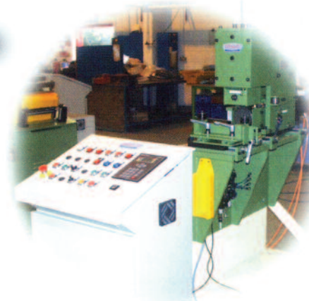
Special Servo Powered Rollfeed for 'Z' Purlins
